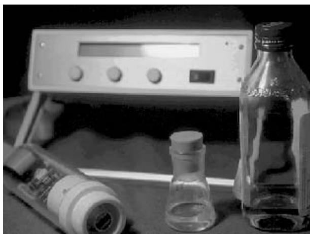
Figure 1.15 The electronic nose. (a) Response of conducting polymer sensor to different concentrations of toluene. (b) Photograph of portable “electronic nose” with an array of conducting polymer sensors (bottom left). (Courtesy of N. Barisci and R. Stella, IPRI, University of Wollongong.)
