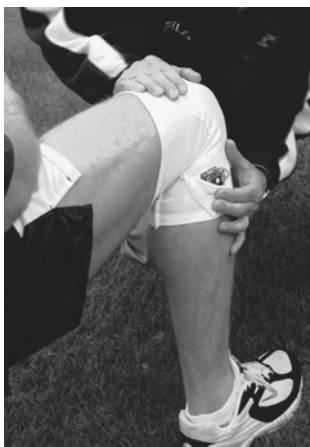
Figure 1.18 Example of fabric strain gauge for determining knee flexion; such devices can be used in sports training, biomechanics studies and rehabilitation.
